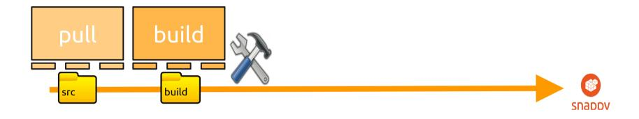
The next step is that each part is built in its parts/part-name/build directory and installs itself into parts/part-name/install.
